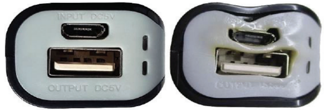
Picture: Which?/ICRT Picture on left shows the USB port of a power bank before the test. Picture on right shows port is melted after the test.
