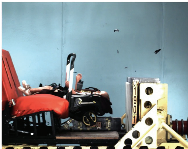
Picture: CNN test of a car seat purchased on an online marketplace that fractured in a 30mph crash test.
