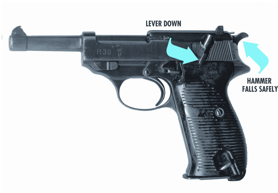
Figure 11: hammer-drop safety deactivates pistol safely while pistol remains loaded; extension of pin above hammer indicates that cartridge is in chamber
