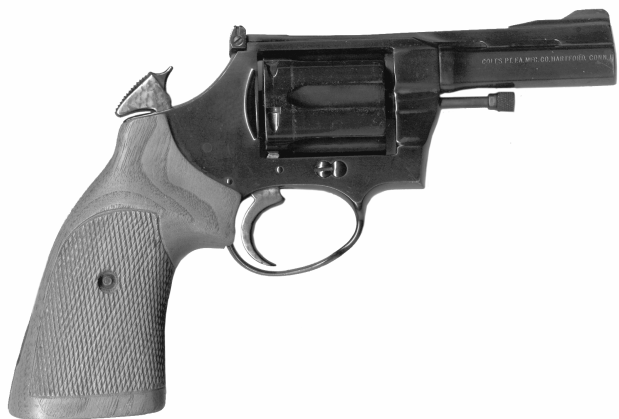
Figure 10: cocked hammer signals revolver ready to fire if loaded
