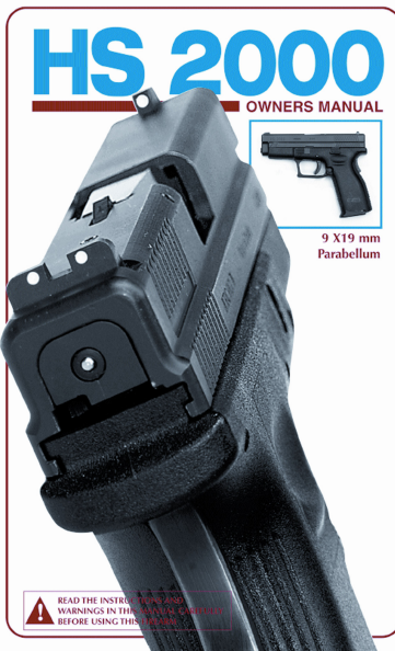
Figure 9: loaded chamber indicator positioned just ahead of rear sight and behind ejection port; ready to fire indicator shows at rear of slide below rear sight. This pistol is loaded and ready to fire
