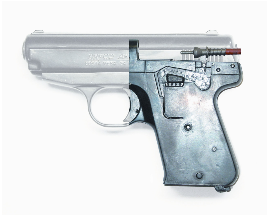
Figure 3: Bryco pistol (phantom view) is equipped with only a single manual safety and cocking indicator
