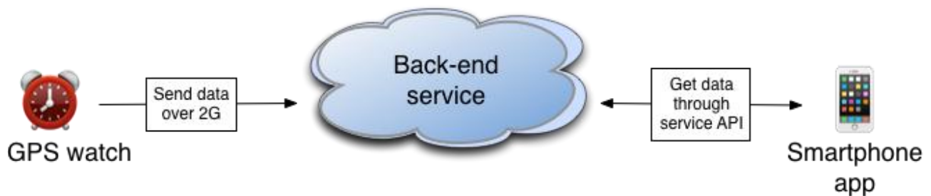
Figure 1. High level data flow between watch, back-end, and app.
